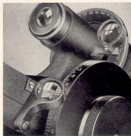
Fig. 14. Magnifying attachment for protractor and power wheel
