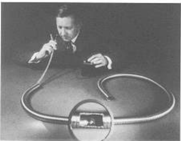
Fiberscope being used to inspect interior of a length of tubing.
