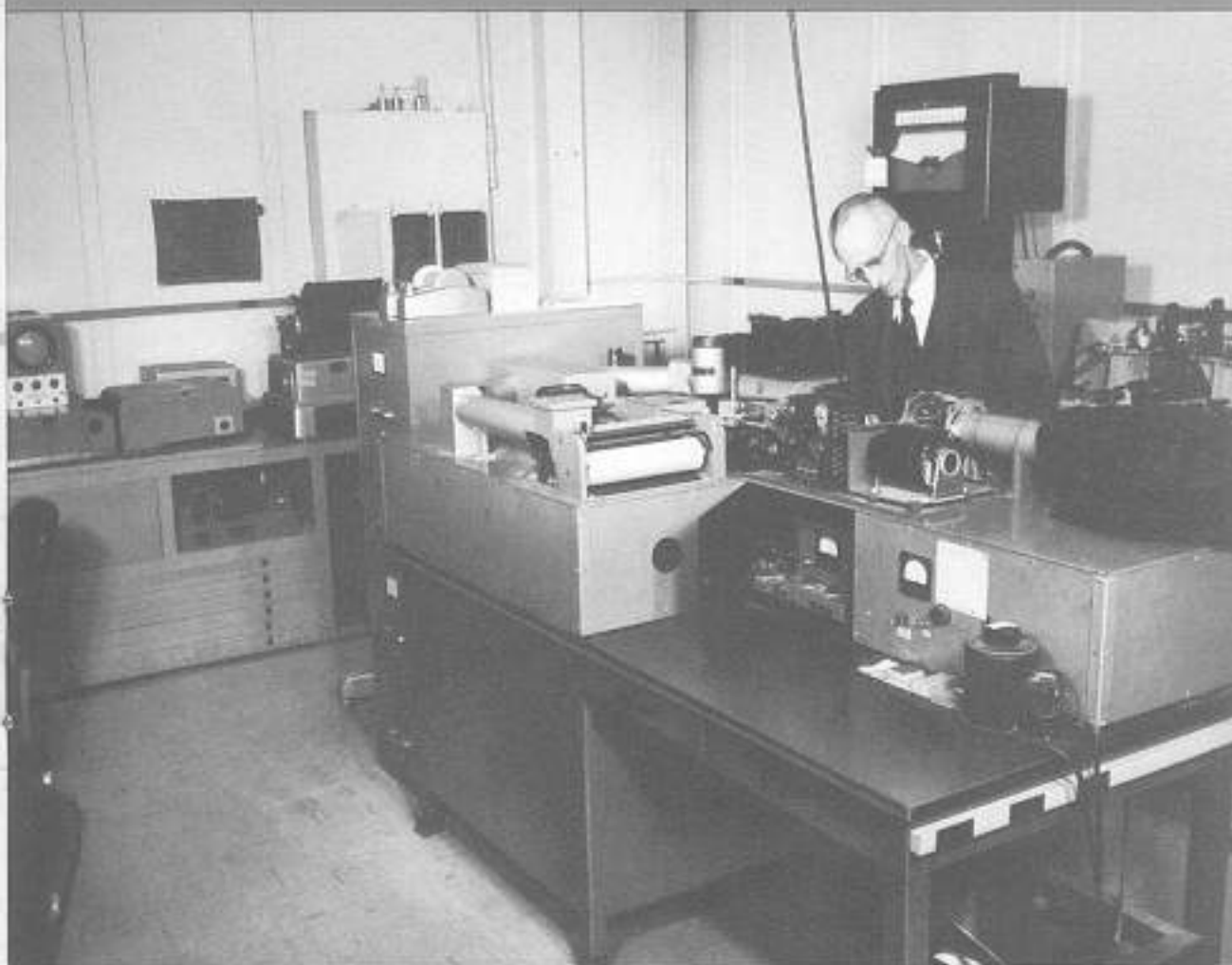
Recording spectrophotometer used for determining transmission characteristics of various substances.
