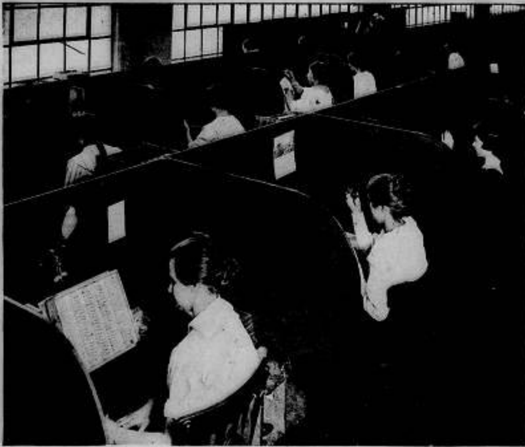
Inspection Booths. The Girls are Trained to Detect the Most Minute Flaw in the Lenses
