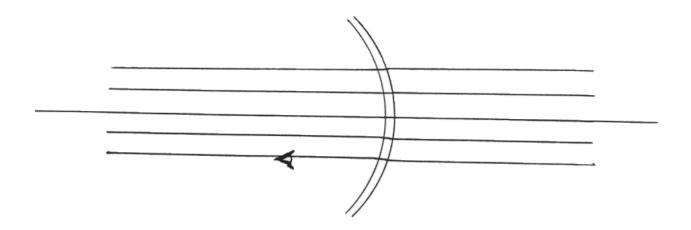
Light entering parallel to the optical axis will exit parallel to that axis. Now, if we think of the eye as being located on one of the emerging rays (not necessarily the optical axis), we see that for straight ahead
