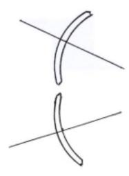
If a large frame were made without face-form, and the lens optical centers located at the wearer's PD, we would again have tilted optical axes:
